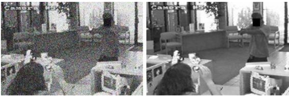
Figure 2. Image with speckle noise (left), and the result of low pass filtering to reduce noise (right).
